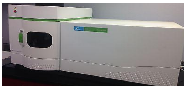
Figure 4. Analysis of sample carried out by Optima 8000 Inductively Coupled Plasma Optically Emitting Spectra (ICP-OES)
