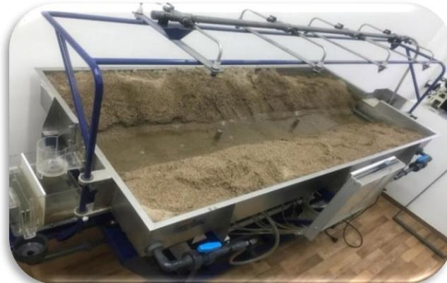
Figure 4. Model of the river channel in the unit
