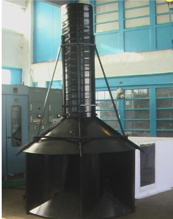
Figure 1 - model of a vortex wind device.
